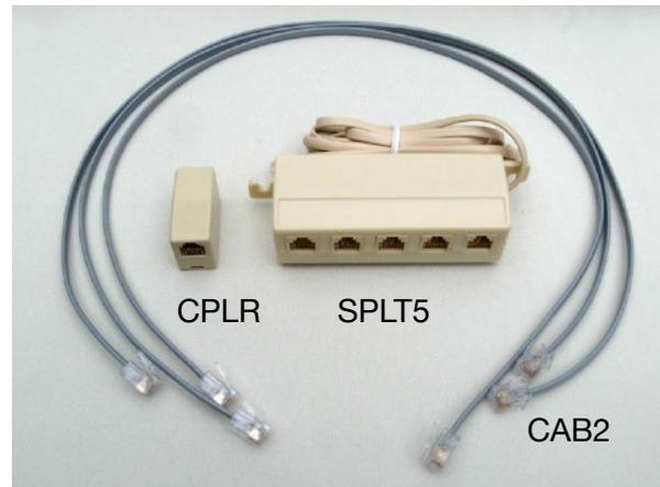
All monitors except the MB5 connect to the PSIU9 with 4-wire telephone cables, couplers, and splitters as shown. Each monitor is supplied with a CAB2 cable (60cm) which connects it to an SPLT5 5-way splitter. The splitters connect to each other in series, and finally through a CPLR coupler and CAB10 cable (305 cm) to the PSIU9.
